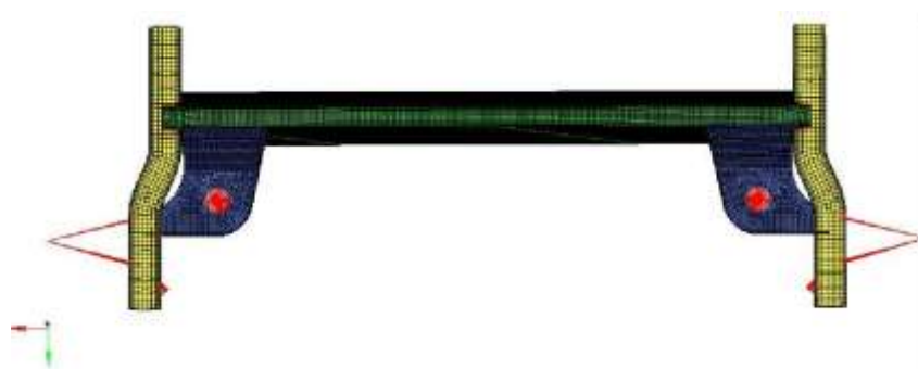
Fig. 2 The finite element model of twist beam
