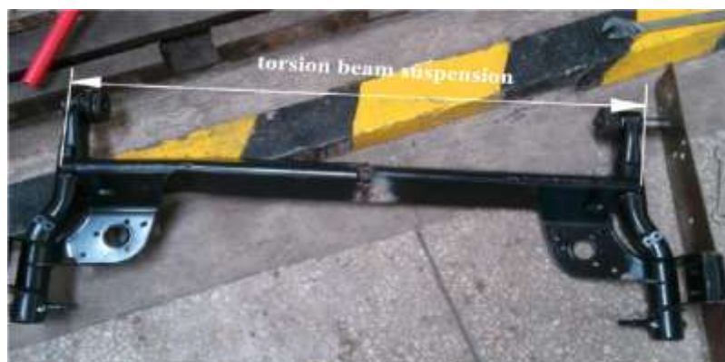
Fig. 1 The Structure of Torsion Beam Suspension
